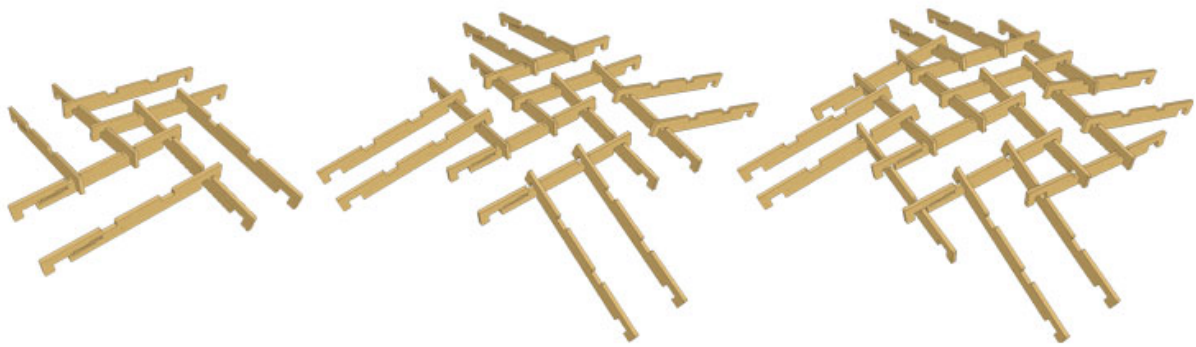
Picture n.2. First steps building a dome in two directions.
